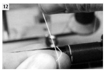
Now unwind one inlay revolution, while leaving the guide wrapping thread where it is, and place the inlay thread underneath and to the right of the guide wrapping thread (8). Allow the oncoming wrapping thread to relax and pin the inlay thread to the blank. At this point the inlay thread should remain under the guide wrapping thread, which has secured it in place.
