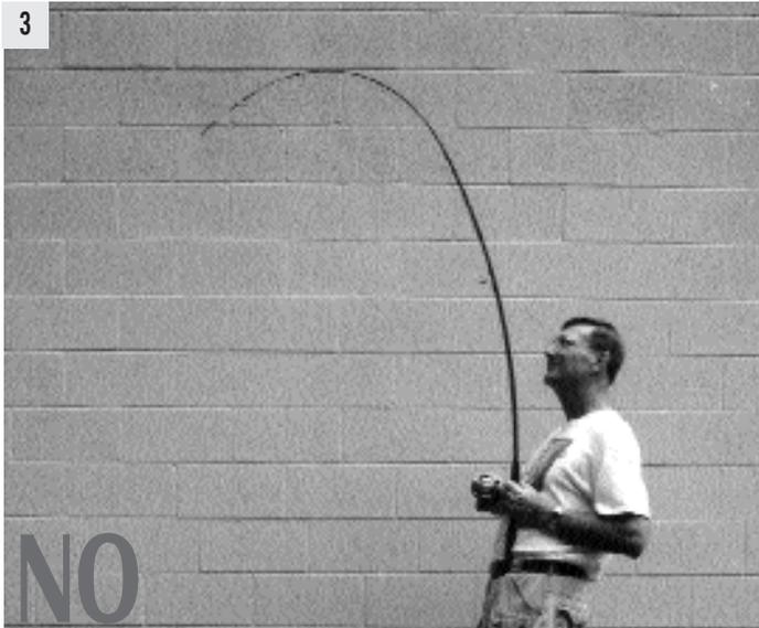
snap off the end of a dry twig. Make sure your customers don't do this to your in-house stock and make sure they understand that there is both a safe and an unsafe way to hand flex a blank.
